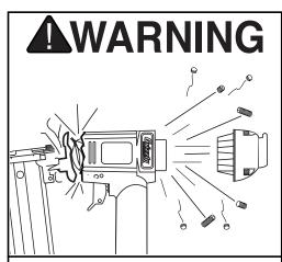
Exceeding the maximum permissible operating pressure may cause the nailer to explode, blowing metal fragments in all directions. To protect yourself from serious personal injury, DO NOT allow your air compressor to exceed the recommended pressure when connected to this nailer!
